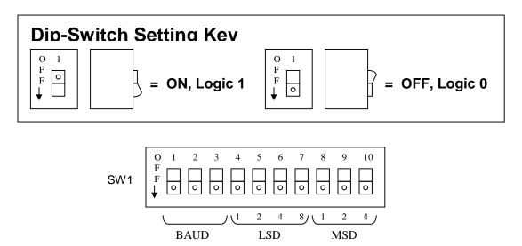
To assign an address of "A" (41h) to the EL=2800, turn on SW1.10 and SW1.4, and leave SW1.5 through SW1.9 in the off position as shown below.
