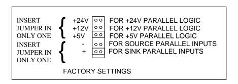
The wiring for the Parallel Data Port is connected to the terminal strip connector TB1 on the parallel interface adapter. TB1 is in two mating halves so the part that the wiring connects to can be removed to connect the wiring and then reinstalled. A copy of the label is shown below.
