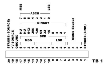
There are four connections required for the MODE SELECT BITS, twelve connections for the BCD or BINARY data bits, or eight connections if the mode is going to be strobed ASCII, and one strobe connection.
