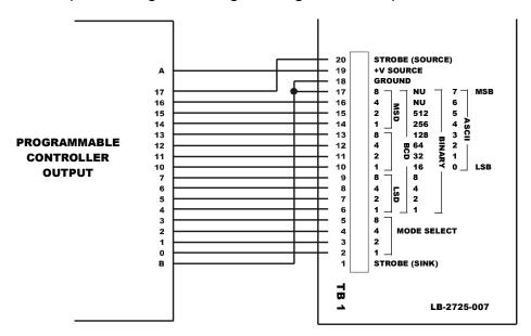
With the above setup, the MODE SELECT bits can be controlled and the mode can be changed as desired. The full range of modes and their functions are shown below. Some modes require a strobe and some do not, as indicated.
